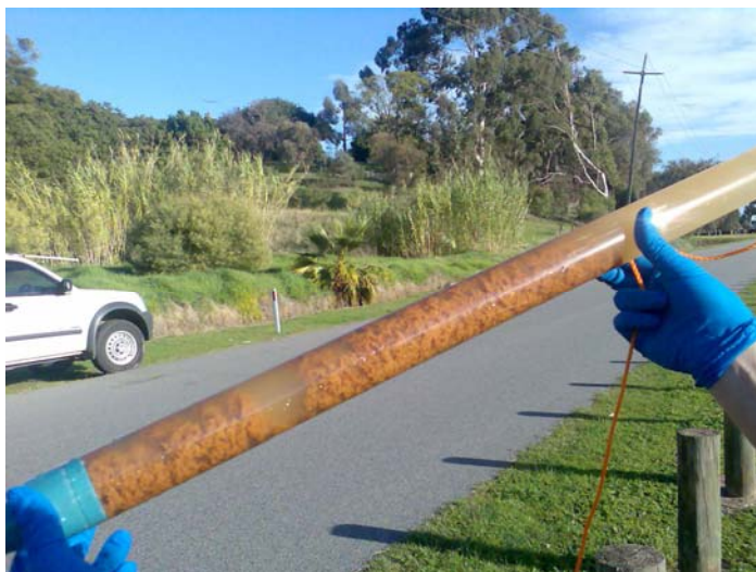
Figure 5: Iron flocculate present in groundwater sampled from CB14
