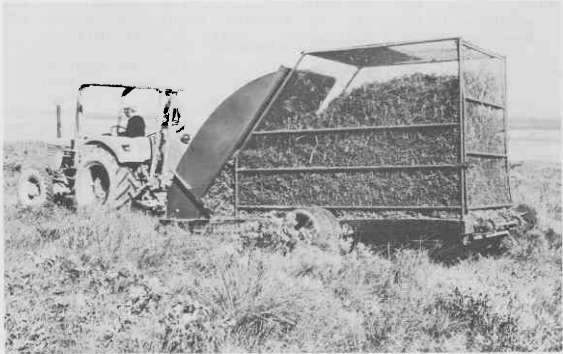
PLATE 1. Grasslands Forage Harvester being used to harvest vegetation from the Western Ti area.
