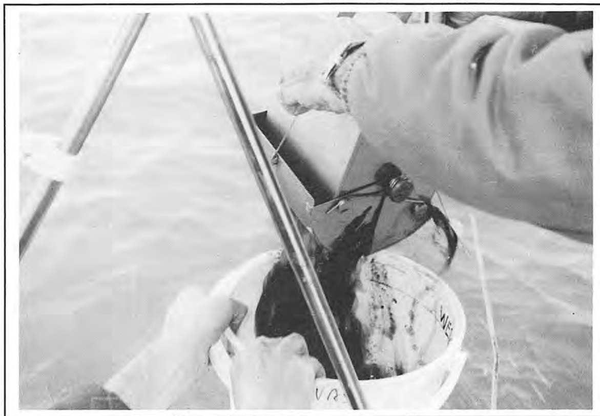
Photograph 24 Harbour sediment being sampled at Bunbury using an Ekman grab for a toxic dinoflagellate cyst survey.
