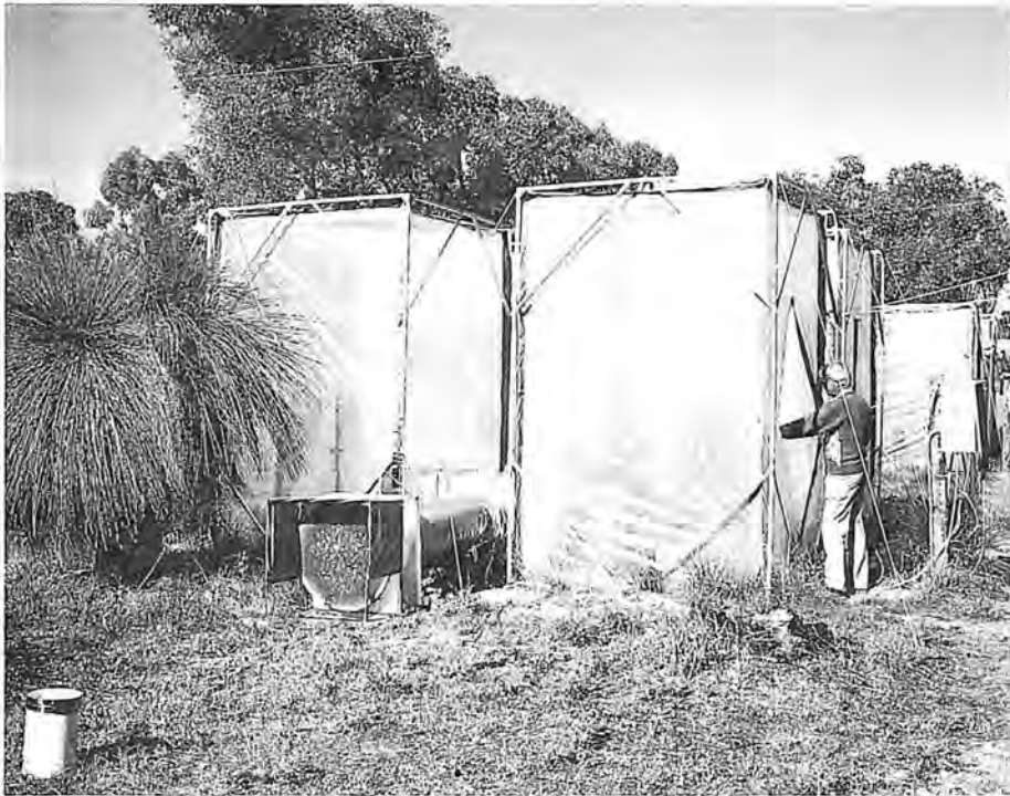
Plate 1. Fumigation canopies, filter, fan and mixer.
