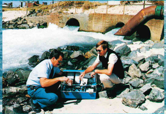
KPCU inspectors collecting waste water from an industrial outfall to be analysed for pollution levels.
