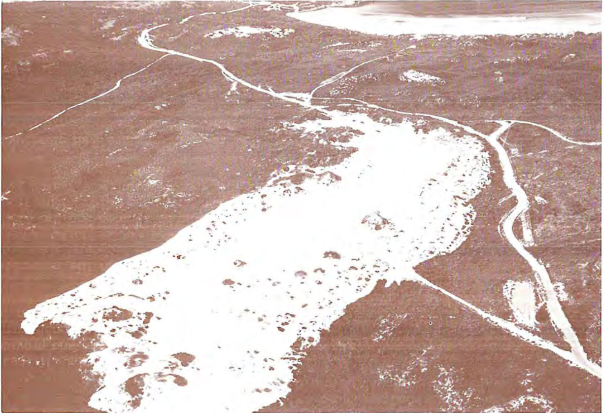
Plate 7. An extensive blow-out associated with a disused quarry in the Sand Dune Unit. This disturbance could have been avoided if proper rehabilitation techniques had been used. (Photo S. Chape)
