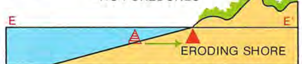
(a & b) Cross sections of the coast following several years of accretion, or erosion (refer Fig. 2).
