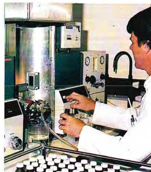
Marine chemist analysing crab flesh on an atomic absorption spectrophotometer for the study on the distribution of contaminants.
