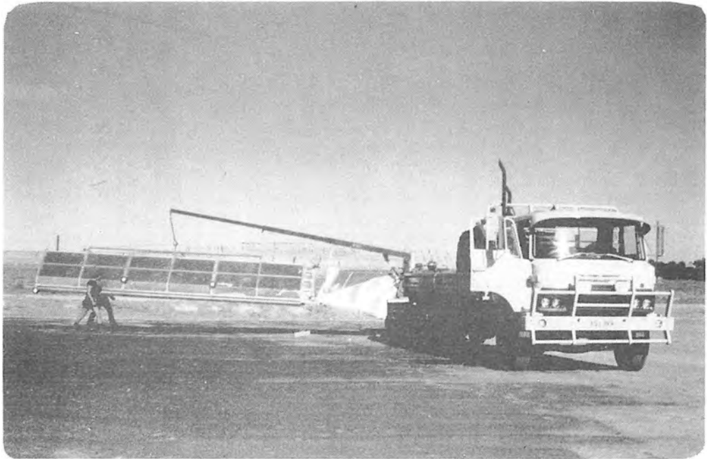
PLATE 19 Portable wind tunnel.
