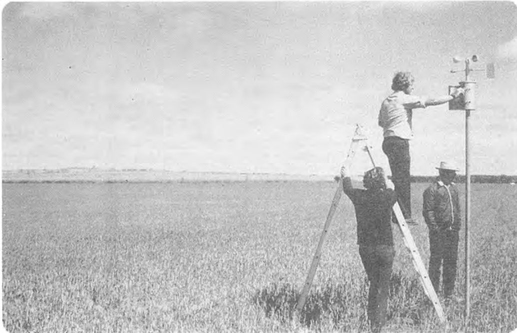
PLATE 24 Maintenance of the Woefle anemometer sited east of the Copperhead slime dumps (in background).
