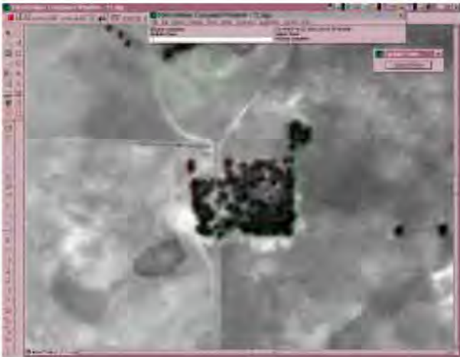
Figure 3.4d: The polygon reflecting the true shape of the remnant patch for 1972 is moved to its original position so that reliable changes are detected when the coverages are overlaid
