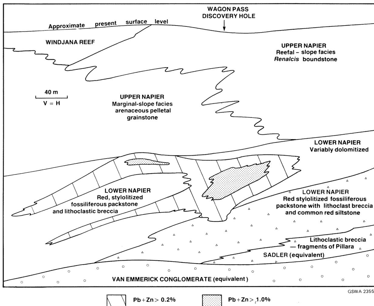
Figure 12. Generalized geological cross-section of the Wagon Pass sulphide ore lens (data courtesy of Shell Co. of Australia Ltd, Metals Division).
