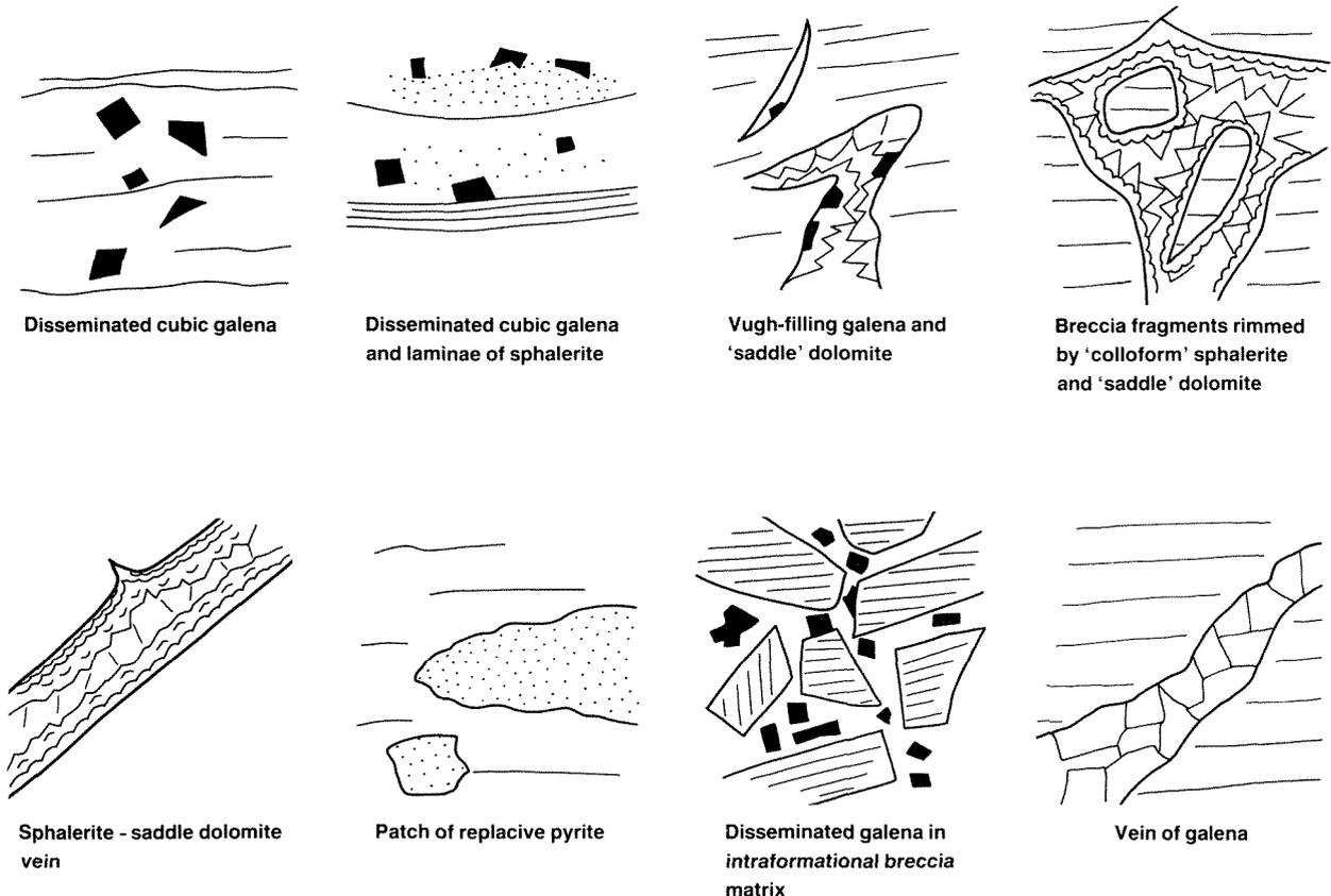
Figure 35. Styles of sulphide mineralization at Sorby Hills (host rock is dolomitized, shaly limestone).
