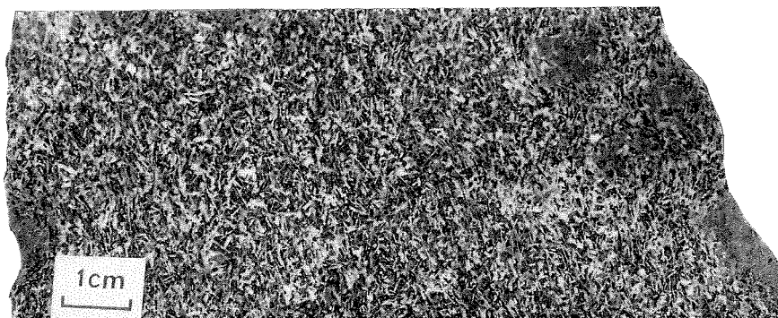
Figure 9. Dark, urutilized (?ortho-)pyroxene phenocrysts displaying glomeroporphyritic texture, in a gabbroic groundmass in which plagioclase exhibits flow alignment, zone 6.
