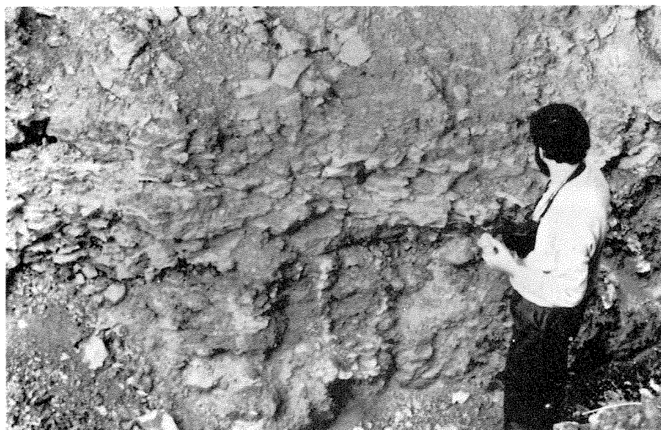
Figure 5. Sheeted silica (silcrete) within poorly cemented nodules.
