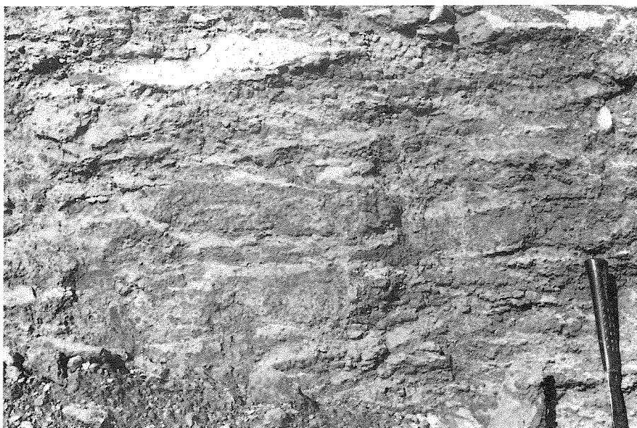
Figure 6. Sheeted carbonate (calcrete) within ferricrete.
