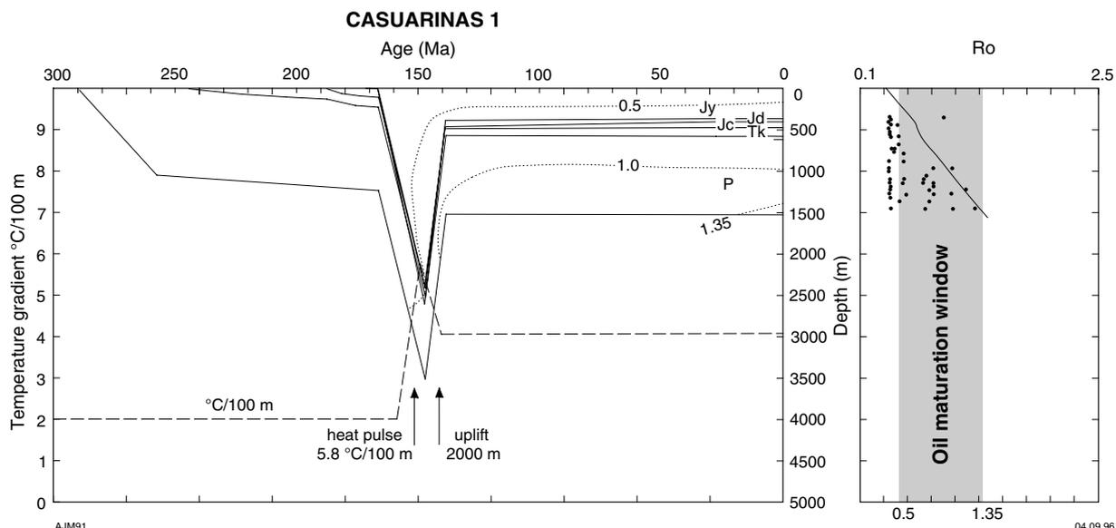
**Figure 52.** Vitrinite reflectance versus depth for Casuarinas 1, showing the large scatter of values. Modelled curve and burial history (time versus depth) plot are also shown. Calculated vitrinite reflectance is the continuous line, and measured samples are represented as dots. Shaded area represents oil window
