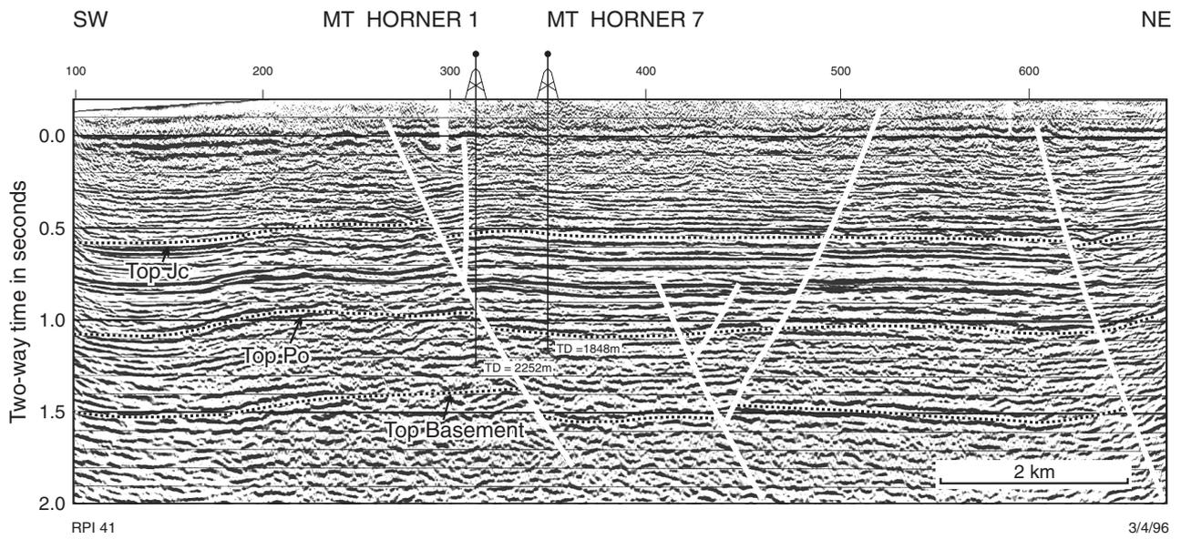
Figure 45. Seismic section (B89-422) showing typical reflection characteristics generated for the top Cattamarra Coal Measures, top Permian, and Precambrian basement horizons
