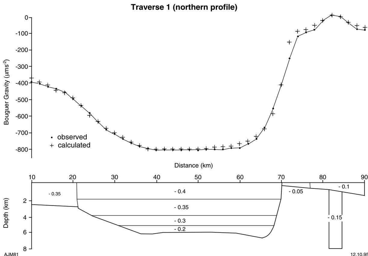
Figure 35. Gravity model for traverse 1 in the northern part of the study area. Calculated and observed Bouguer gravity are in  $\text{mm/sec}^2$  and density is shown in  $\text{g/cm}^3$ . Distance along traverse and depth of body are in kilometres
