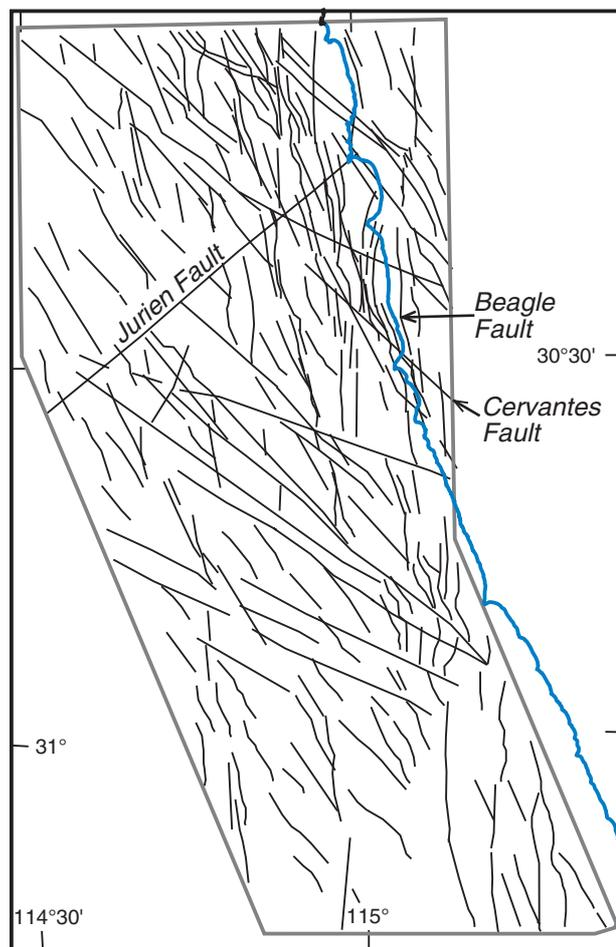
**Figure 41.** Major aeromagnetic lineaments in the Wedge Island–Jurien area WA-228-P (from Heath et al., 1994 — digital data supplied Woodside Offshore Petroleum)
