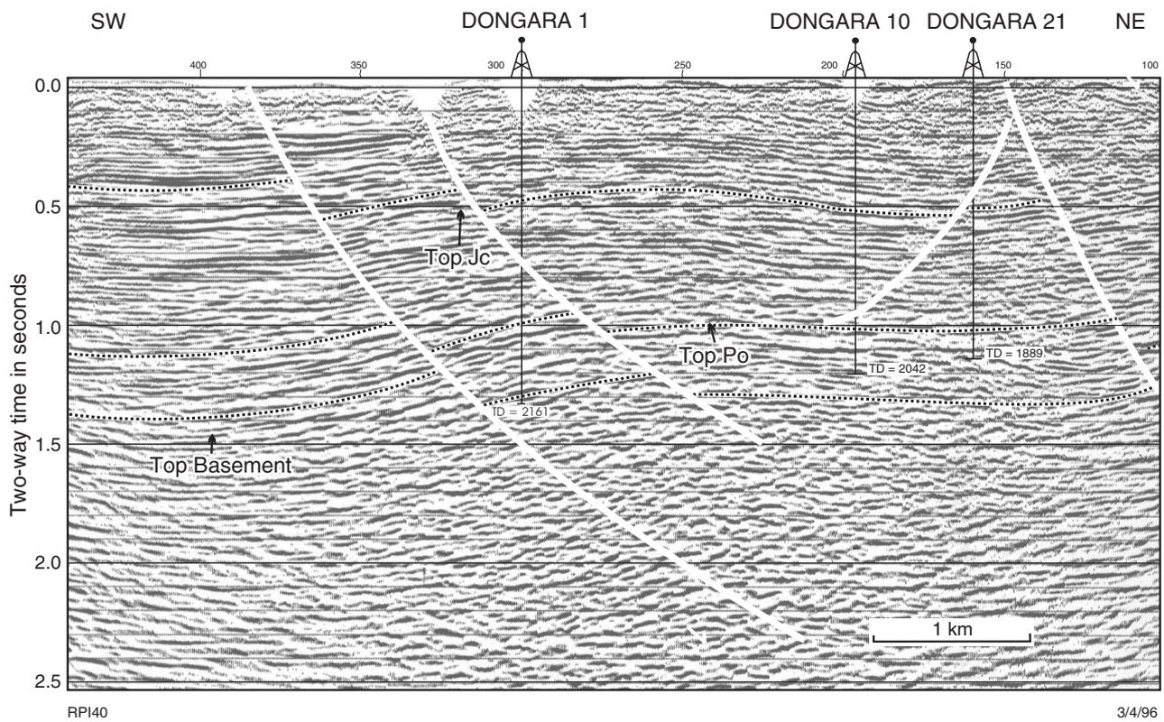
Figure 46. Seismic section (P89-01L) across the Dongara field showing the variable nature of basement-horizon reflection characteristics
