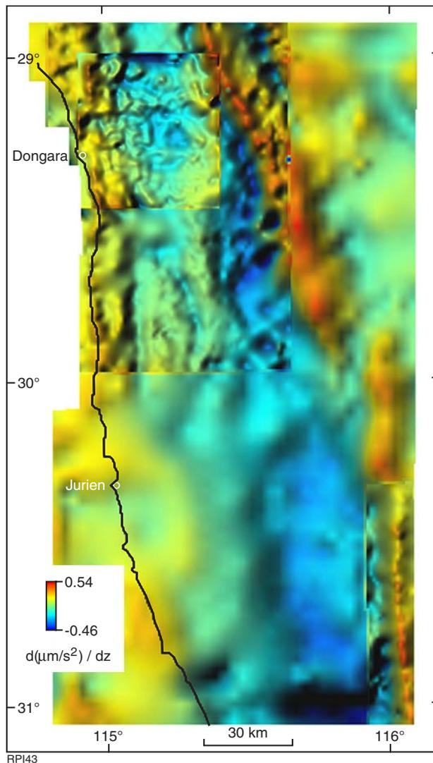
Figure 30. Gravity image of first vertical derivative for the northern Perth Basin. Sun illumination 80 degrees from the northwest. Note that the data is aliased in the southwest of the image
