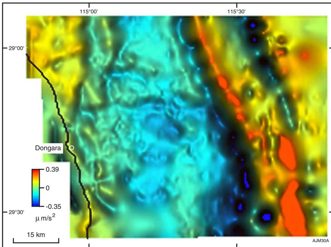
Figure 32. First vertical derivative gravity image for the Dongara–Mount Horner area. Sun illumination 60 degrees from the northwest
