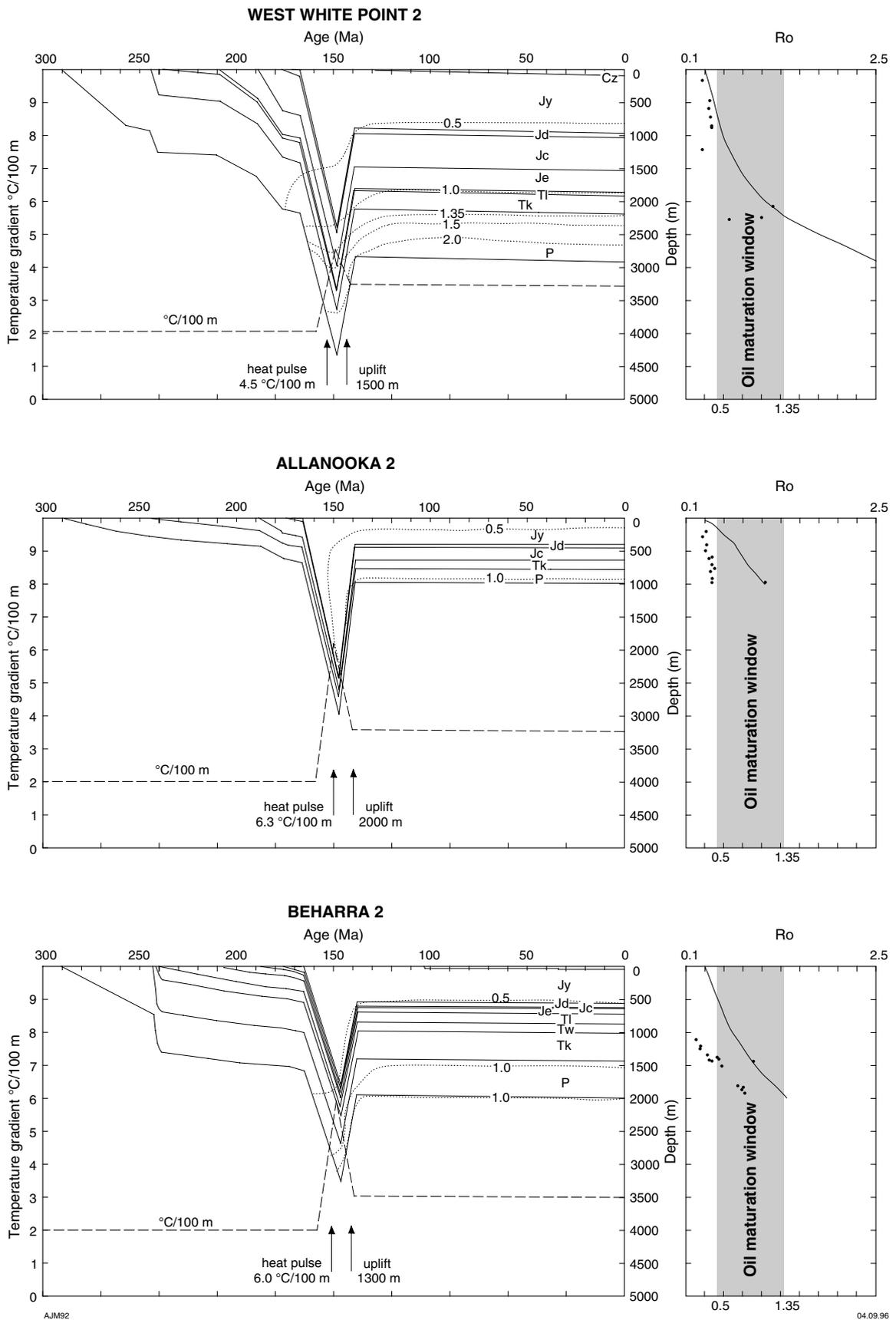
Figure 53. Vitrinite reflectance versus depth for West White Point 2, Allanooka 2, and Beharra 2, including burial history (time versus depth) plot. Calculated vitrinite reflectance is the continuous line, and measured samples are represented as dots. Shaded area represents oil window
