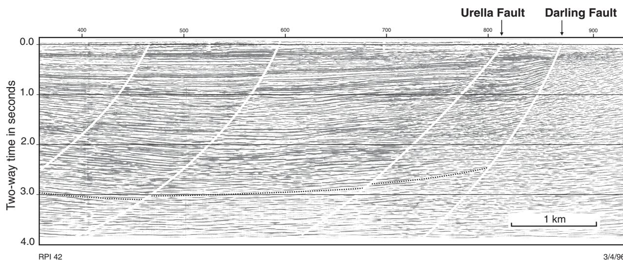
Figure 48. Seismic section (A89-708) showing the character of the Darling Fault
