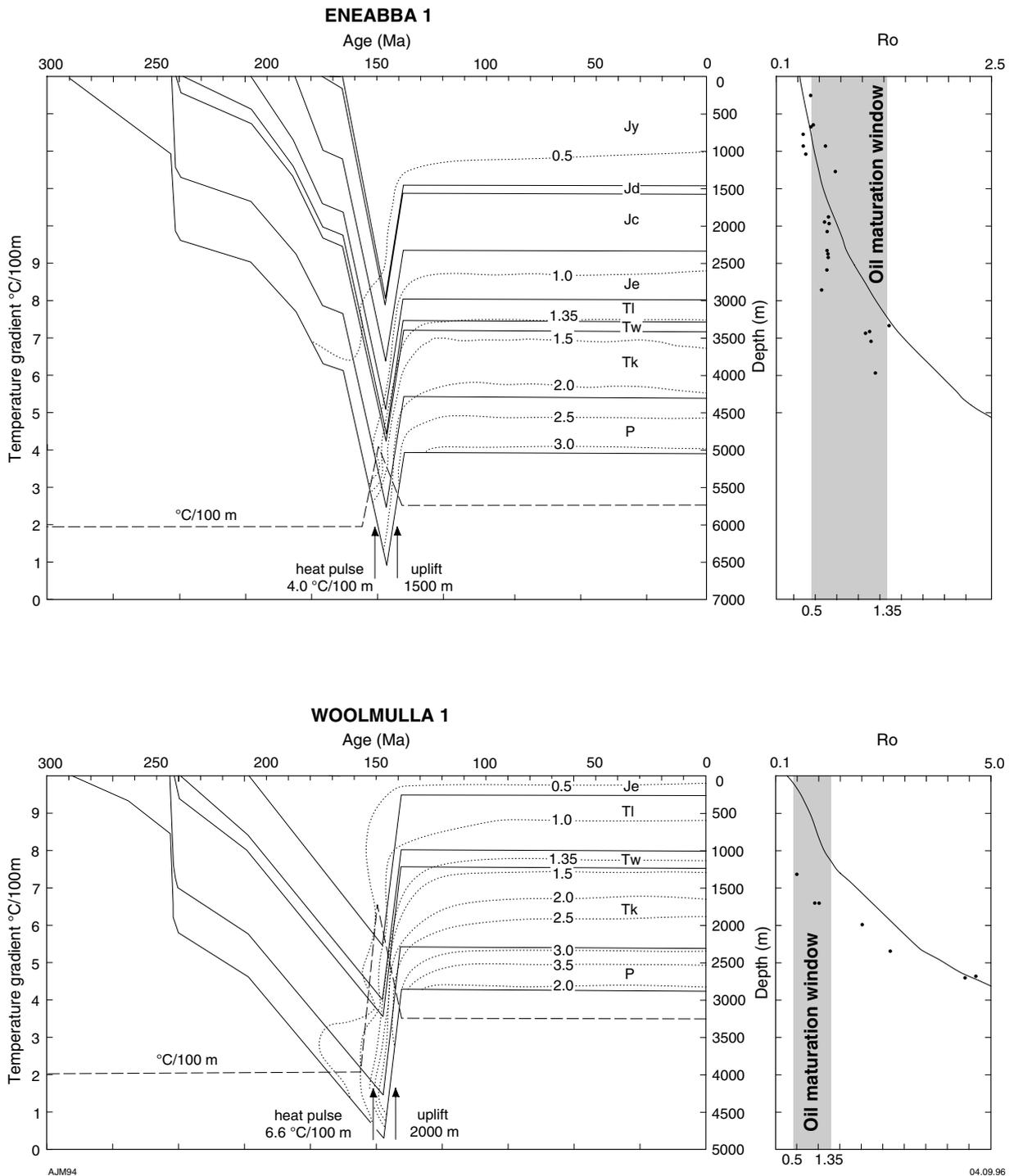
**Figure 55. Vitrinite reflectance versus depth for Eneabba 1 and Woolmulla 1, including burial history (time versus depth) plot. Calculated vitrinite reflectance is the continuous line, and measured samples are represented as dots. Shaded area represents oil window**
