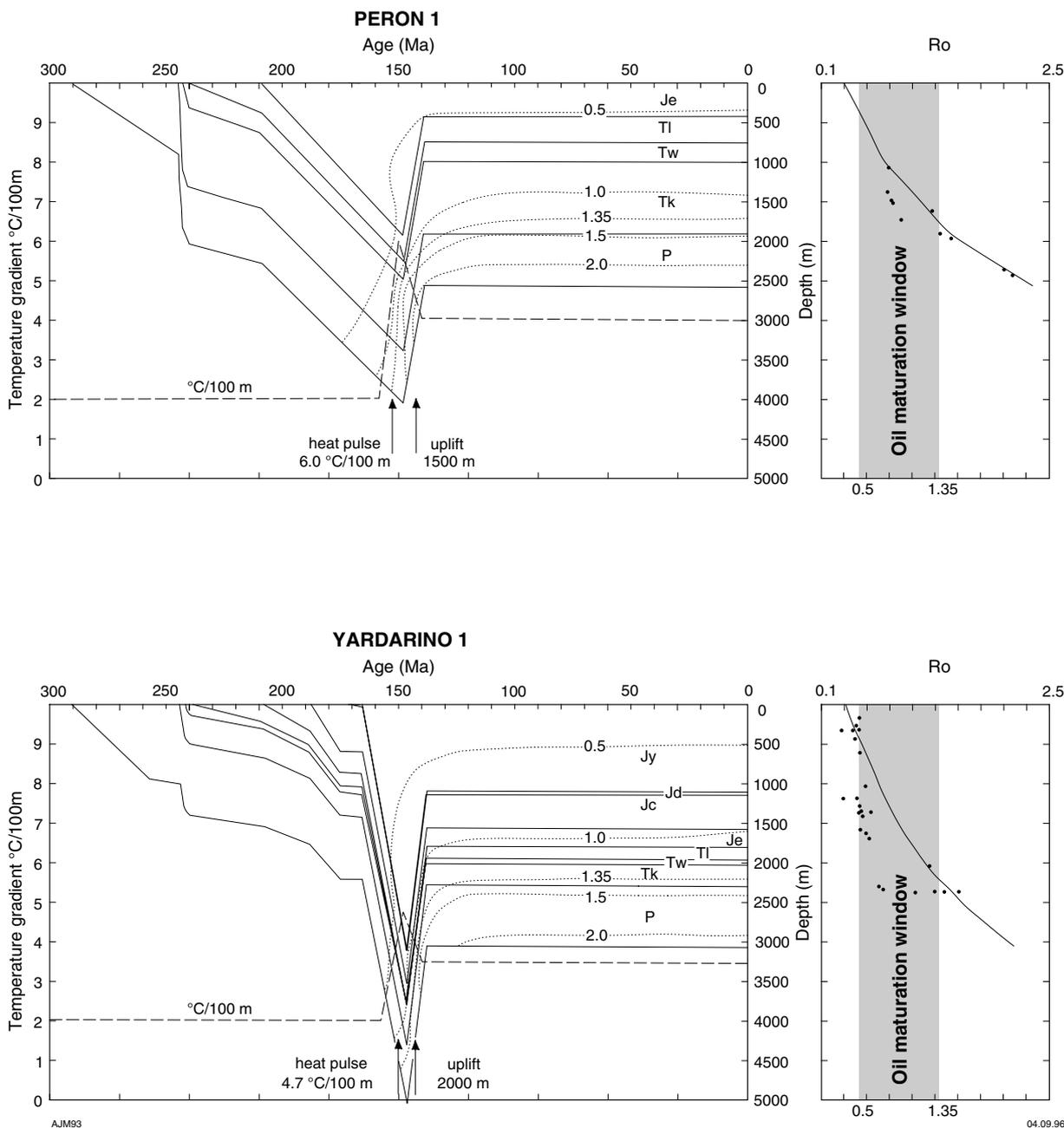
Figure 54. Vitrinite reflectance versus depth for Peron 1 and Yardarino 1, including burial history (time versus depth) plot. Calculated vitrinite reflectance is the continuous line, and measured samples are represented as dots. Shaded area represents oil window
