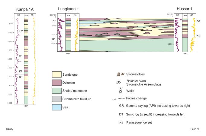
Figure 12. Depositional model for the Kanpa Formation in the Yowalga area (after Apak and Moors, 2000a): a) model showing carbonate and siliciclastic cycles within shallow-marine to lagoonal and sabkha environments; b) sequencestratigraphic correlation showing the lateral facies distribution between Hussar 1, Lungkarta 1, and Kanpa 1A
