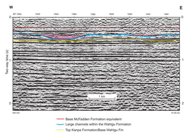
Figure 14. Seismic line N83-8 showing deep channels, which incised into the Steptoe Formation, within the Wahlgu Formation. For location of seismic line see Figure 7
