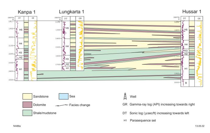
Figure 11. Depositional model for the Hussar Formation in the Yowalga area (after Apak and Moors, 2000a): a) model showing a very low relief basinal setting with multiple prograding carbonate and siliciclastic cycles; b) sequence-stratigraphic correlation showing the lateral facies distribution between Hussar 1, Lungkarta 1, and Kanpa 1A
