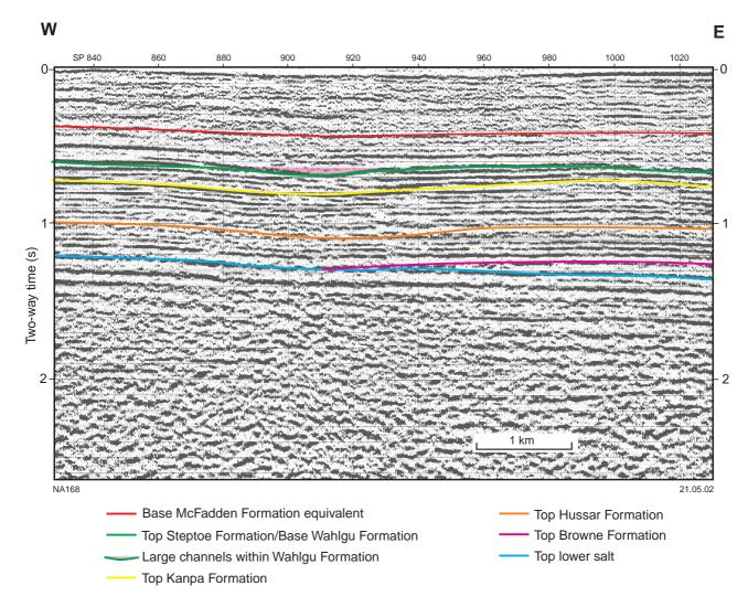
Figure 13. Seismic line N83-11 showing a channel incised into the Steptoe Formation. For location of seismic line see Figure 7
