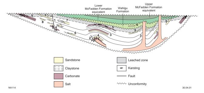
Figure 29. Schematic petroleum play types present in the Gibson area: 1) normal fault trap; 2) drape over salt high; 3) lateral salt seal; 4) fractured reservoir; 5) leach-enhanced porosity; 6) pinchout traps; 7) lateral facies change; 8) erosive channel or valley
