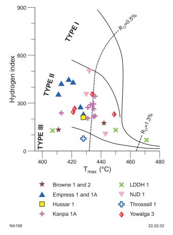
Figure 24. Kerogen type as a function of T<sub>max</sub> versus hydrogen index from Rock-Eval pyrolysis (after Ghori, 2000)
