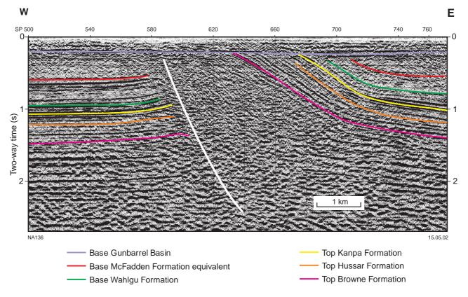
Figure 19. Seismic line N83-7 showing late-stage salt emplacement and erosion of Supersequence 1 strata, Wahlgu Formation, and McFadden Formation equivalent. For location of seismic line see Figure 7
