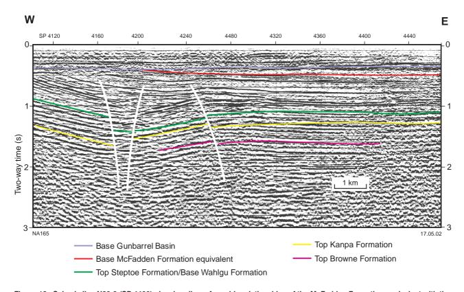
Figure 18. Seismic line N83-2 (SP 4400) showing disconformable relationships of the McFadden Formation equivalent with the Wahlgu Formation below, and the Table Hill Volcanics above. For location of seismic line see Figure 7
