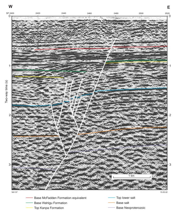
Figure 21. Seismic line N83-6 showing late strike-slip faulting event post-dating the Wahlgu Formation and displaced base McFadden Formation equivalent unconformity. Note that the Steptoe Formation was eroded on the upthrown side of the fault block. For location of seismic line see Figure 7
