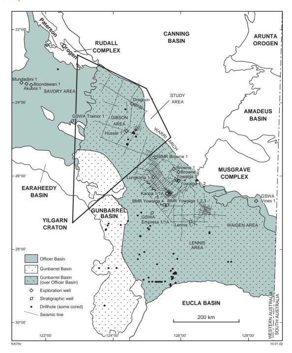
Figure 3. Location of petroleum exploration wells, stratigraphic tests, mineral exploration drillholes, and complete seismic coverage over the Officer Basin
