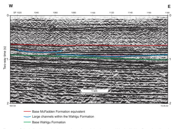
Figure 15. Seismic line N83-7 showing very large channel development within the Wahlgu Formation. Note the potential seal at the top of channels. For location of seismic line see Figure 7
