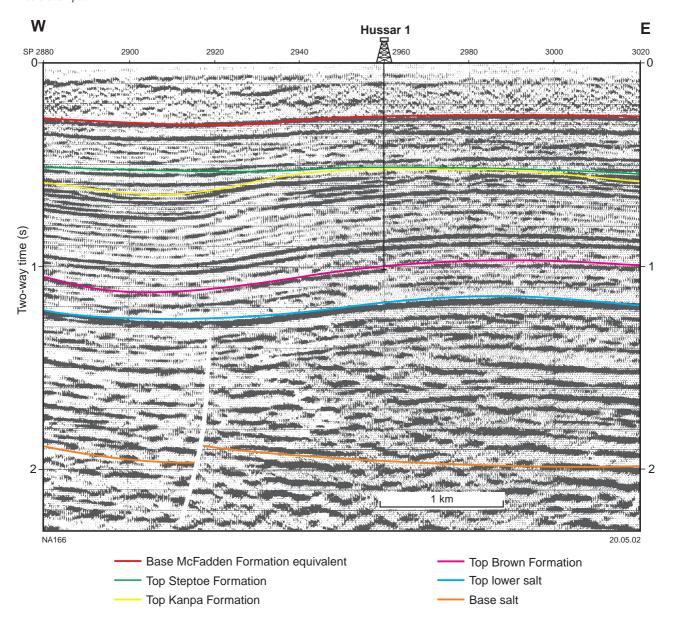
Figure 8. Seismic line N83-6 showing Hussar 1 structure and the absence of the Steptoe Formation. Note that the Kanpa Formation is overlain unconformably by the Wahlgu Formation (previously called as McFadden Formation). The McFadden Formation equivalent is also assigned to the unnamed unit that overlies the Wahlgu Formation in this well
