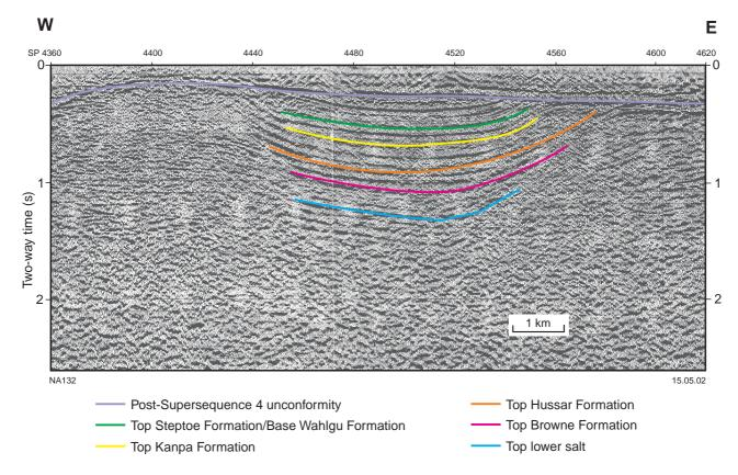
Figure 9. Seismic line N83-3A showing a residual of Supersequence 1 and Wahlgu Formations between the salt emplacements. For location of seismic line see Figure 7
