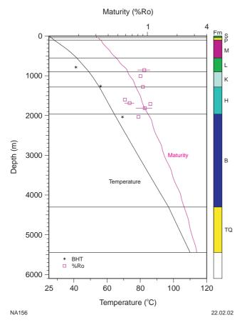
Figure 25 Measured and modelled temperature and thermal maturity in Hussar 1. The sedimentary sequences indicated on this figure are the Samuel Formation (S), Paterson Formation (P), McFadden Formation equivalent (M), Lennis Sandstone (L), Kanpa Formation (K), Hussar Formation (H), Browne Formation (B), and Townsend Quartzite (TQ)
