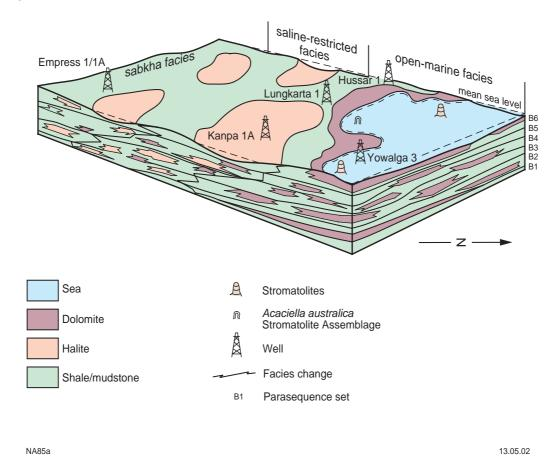
Figure 10. Depositional model for the Browne Formation in the Yowalga area (after Apak and Moors, 2000a) showing a large, flat basin with numerous shallow ponds flooded during storms, a sequence-stratigraphic correlation, and the lateral facies distribution within the formation.
