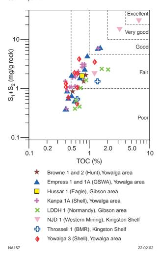
Figure 23 Petroleum generating potential as a function of organic richness versus potential yield for samples interpreted as reliable (after Ghori, 2000)
