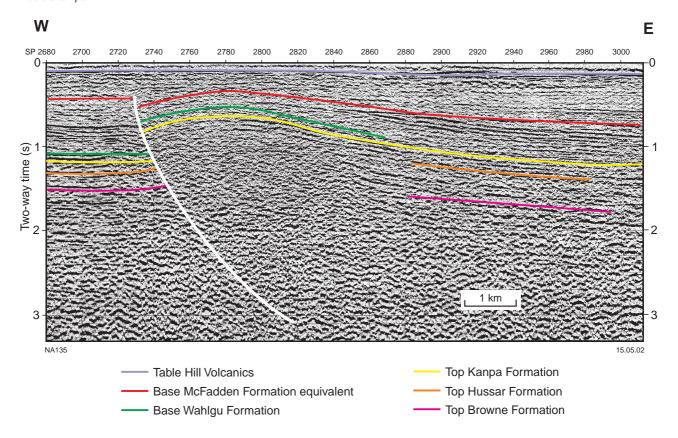
Figure 17 Seismic line N83-11 showing an angular unconformity between the Wahlgu and the McFadden Formation equivalent.
