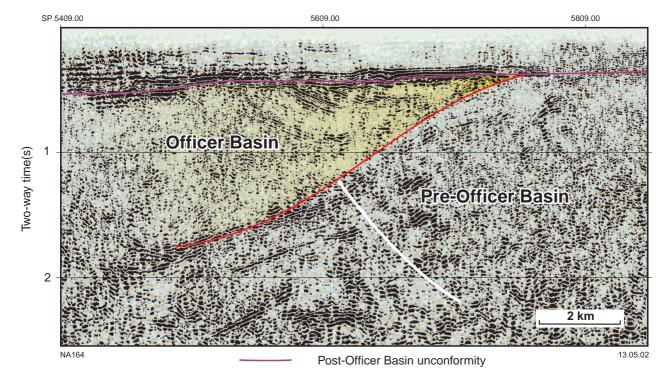
Figure 4. Seismic line N83-3A showing the relationships between the Neoproterozoic Officer Basin and an underlying Mesoproterozoic basin. For location of seismic line see Figure 7
