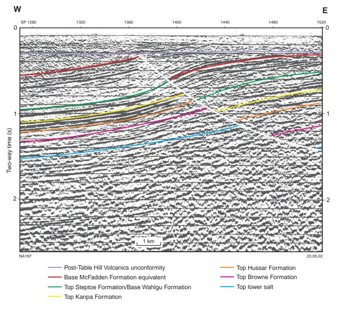
Figure 20. Seismic line N83-7 showing late faulting event post-dating the McFadden Formation equivalent. Faulting event resulted in significant displacement of Supersequence 1 strata, Wahlgu Formation, and McFadden Formation equivalent. The McFadden Formation equivalent was eroded and later covered by the younger Gunbarrel Basin strata. For location of seismic line see Figure 7
