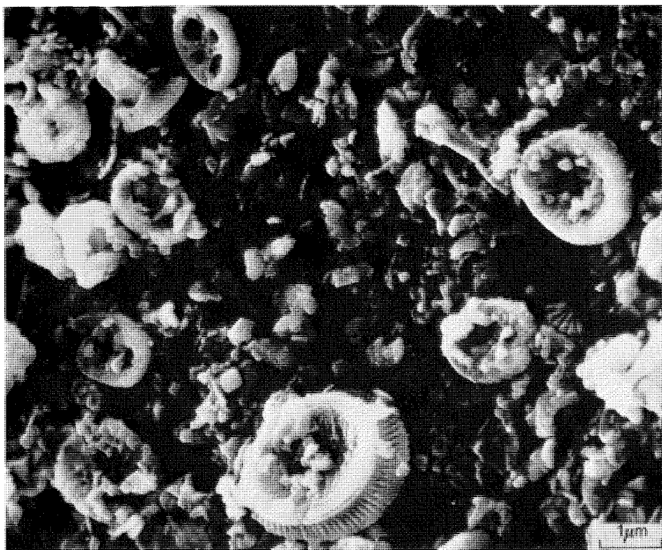
Figure 40. Scanning electron microscope photograph of Gingin Chalk showing abundant coccoliths. Photograph by courtesy of West Australian Petroleum Pty Ltd.
