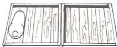
Undersurface of the device showing the framework upon which the boards are mounted, and the plastic water bottle in place.
