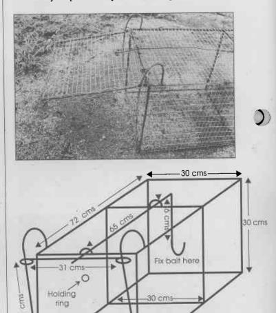
Bait taken, ring released, barrier drops to base and holds door closed.
