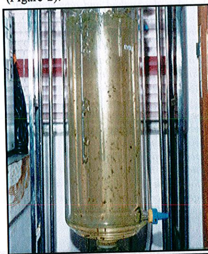
Fig. 2: Somatic embryo production in bioreactor
