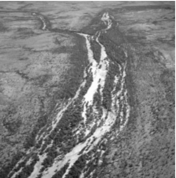
Upper Ord River, Kimberley. Mix of braided characteristics (unstable bars, abundant sand bedload, high width/depth ratio) and anabranching characteristics (some stable, vegetated, linear islands separating multiple, interconnected channels). Fairly straight form at reach to subcatchment scale.
