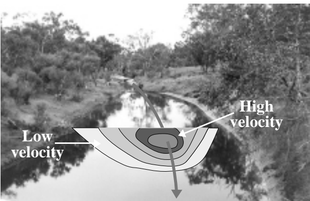
Figure 16. The path of high velocity flow.
