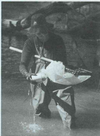
Jane Growsns sampling snags in the Campaspe River with the snag bag, a simple yet effective devise designed to overcome the difficulty of sampling snags in lowland rivers.
