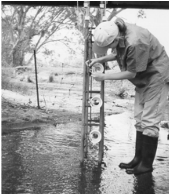
A suspended sediment sampler is used to detect the amount of sand in a water sample
