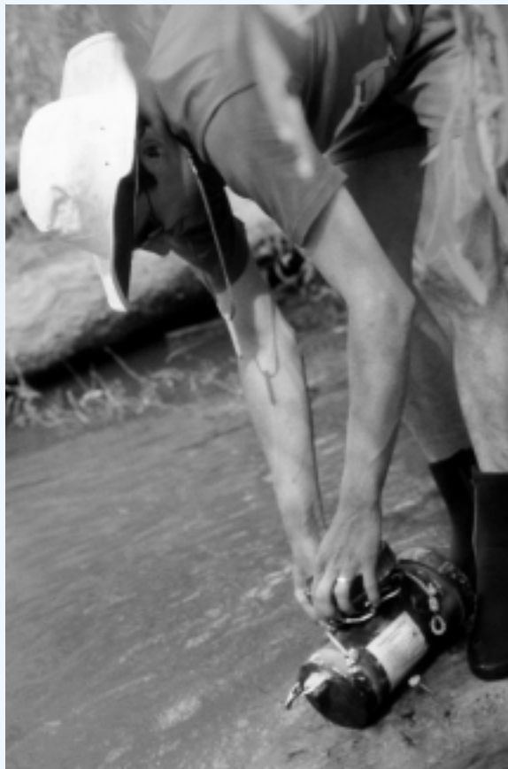
Simon Treadwell attaching the perspex chamber used to measure production of biofilms on snag surfaces. Photo: Ben Gawne
