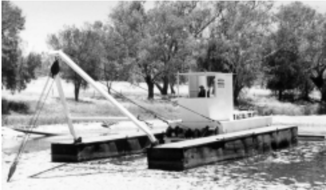
Photos showing the accumulation of sediment in Burlong Pool near Northam. The dredge is used to excavate sand with an estimated 10,000m 3 being removed from Burlong Pool annually.
