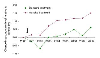
Fig. 2. Change in observed valley groundwater levels from the water levels predicted to occur if there was no treatment. A positive value indicates a rise in water level relative to the control. Arrow shows time of treatment.
