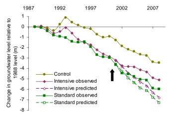
Fig. 1. Change in groundwater levels in treated and control catchments relative to 1988 level (solid symbols) and predicted change in groundwater levels in treated catchments relative to control if there was no treatment (open symbols). Arrow shows time of treatment.
