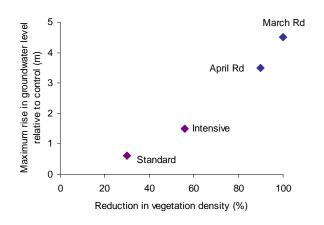
Fig. 3. Change in valley groundwater levels relative to control, in response to reduction in vegetation density, in this study compared with treatments in use in the 1970s and 80s (April Rd, March Rd).
