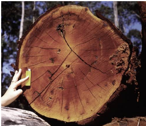
Cross section of karri billet showing borer infestation and associated brown wood staining.
