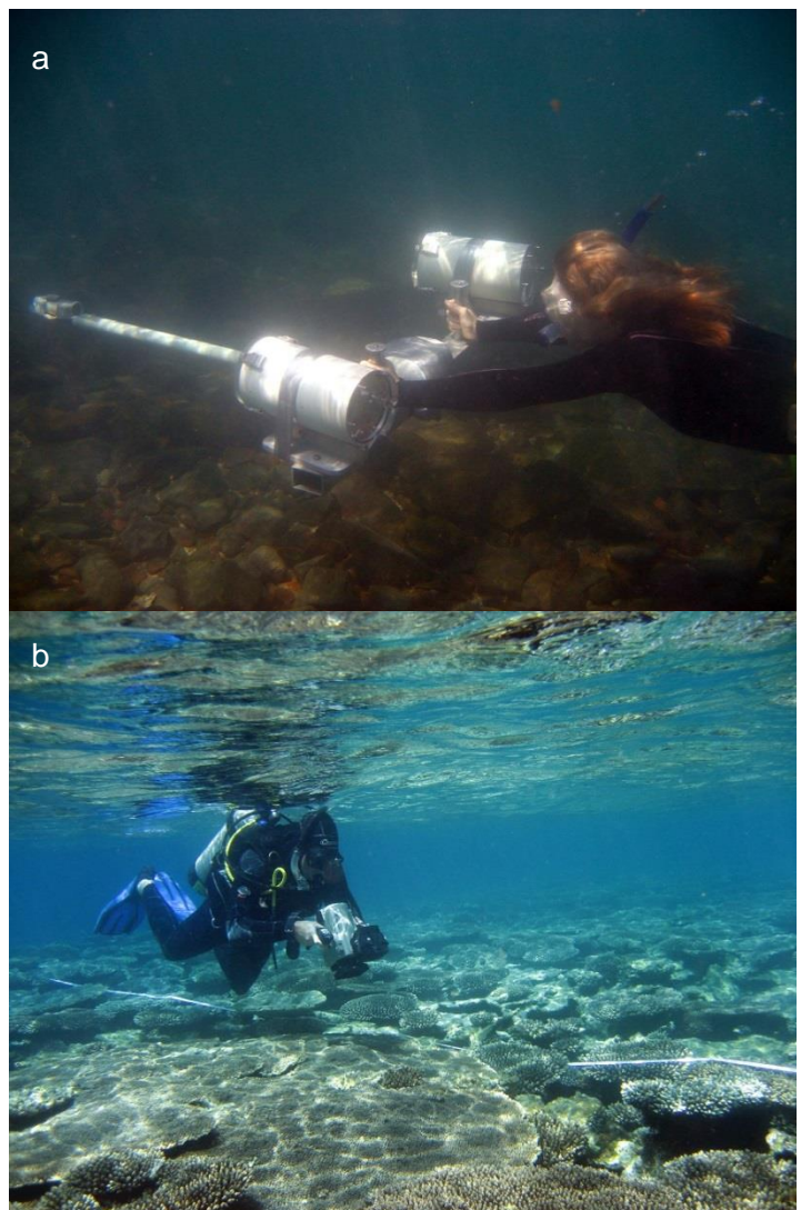
Above: Marine scientists collecting fish survey data using stereo-diver operated video (a) and capturing benthic images for photo quadrats to assess benthic assemblages (b).
