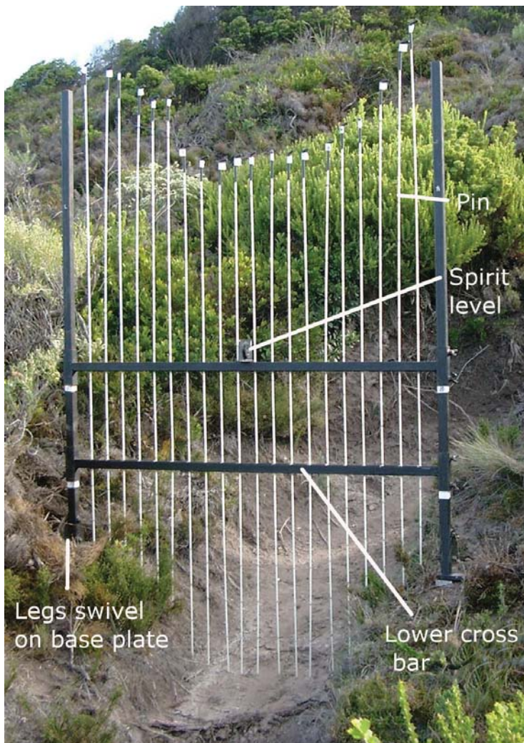
Figure 6. PIN frame erected in situ (Bald Head trail) showing the pins reading the cross sectional trail profile.
