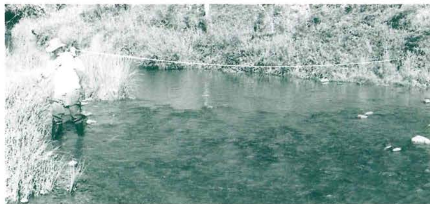
Above: Measuring stream width on Adelong Creek as part of PBH habitat assessment.
