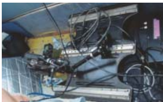
Top: Beechcraft Barron used for aerial video survey. Above: Camera setup through the floor of the plane.
