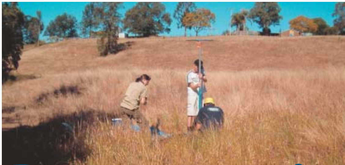
Collecting soil samples for measuring denitrification potential outside the riparian zone at Sandy Creek, Qld. Photo Carol Conway.
