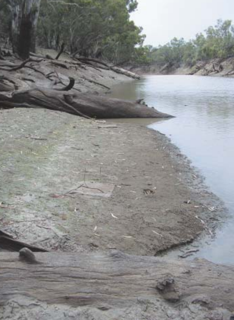
Above: A low level inset-floodplain on the Bourke reach of the Barwon Darling River, showing two sediment mats used to collect sediment deposited during inundation. Photo Mark Southwell.
