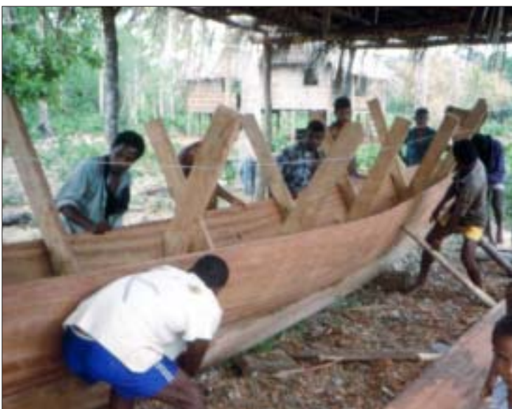
Figure 7. Keel log with frames attached, and first plank being fitted. (M. Smaalders 1997)
