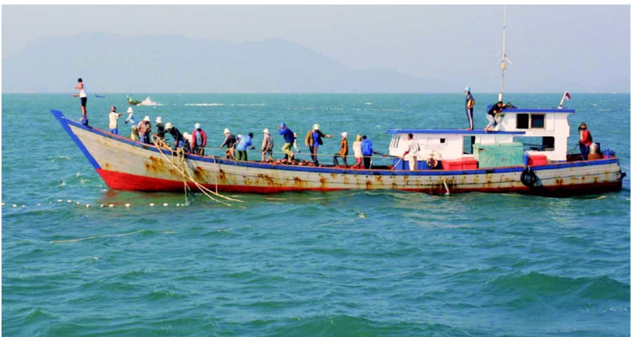
Figure 3. A purse-seine boat closing the bottom of the net.
