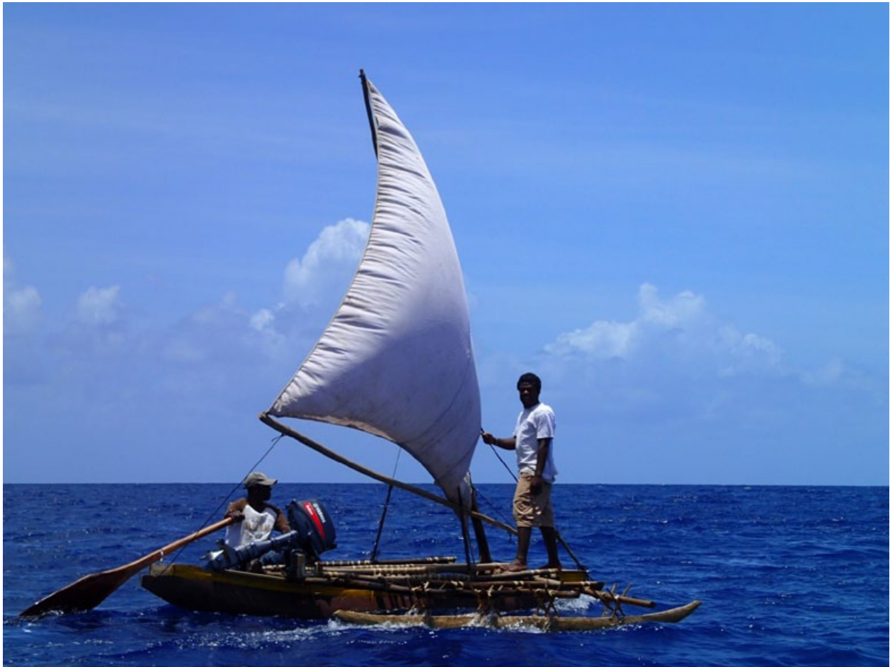
Photo 7. Sea trials of the “modified canoe” demonstrated that with a good wind local fishermen do not need to rely on outboard engines.
