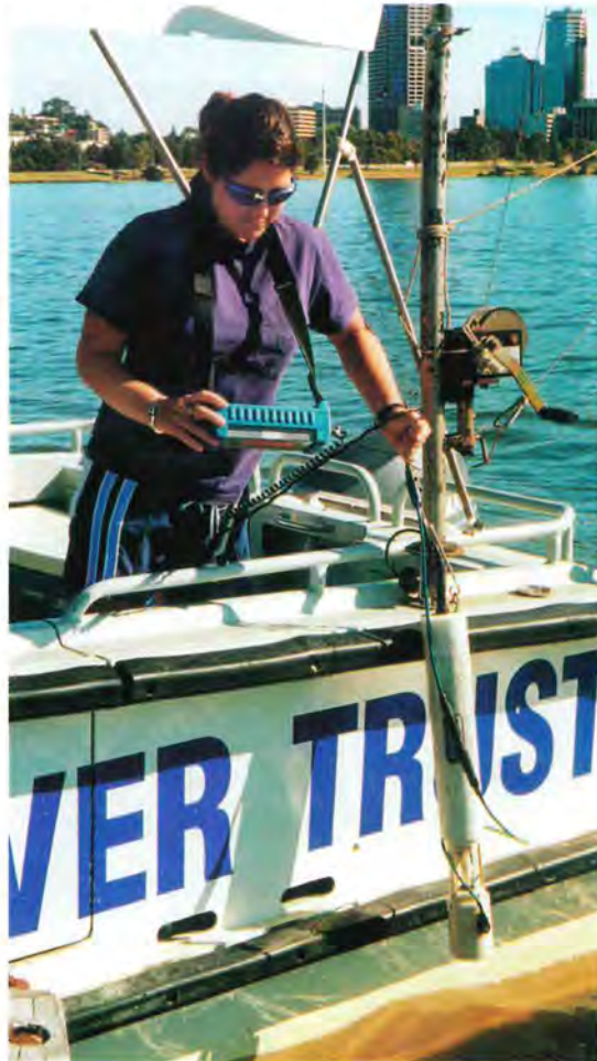
Water and Rivers Commission employee Amanda Wilson taking physical measurements with a hydrolab
