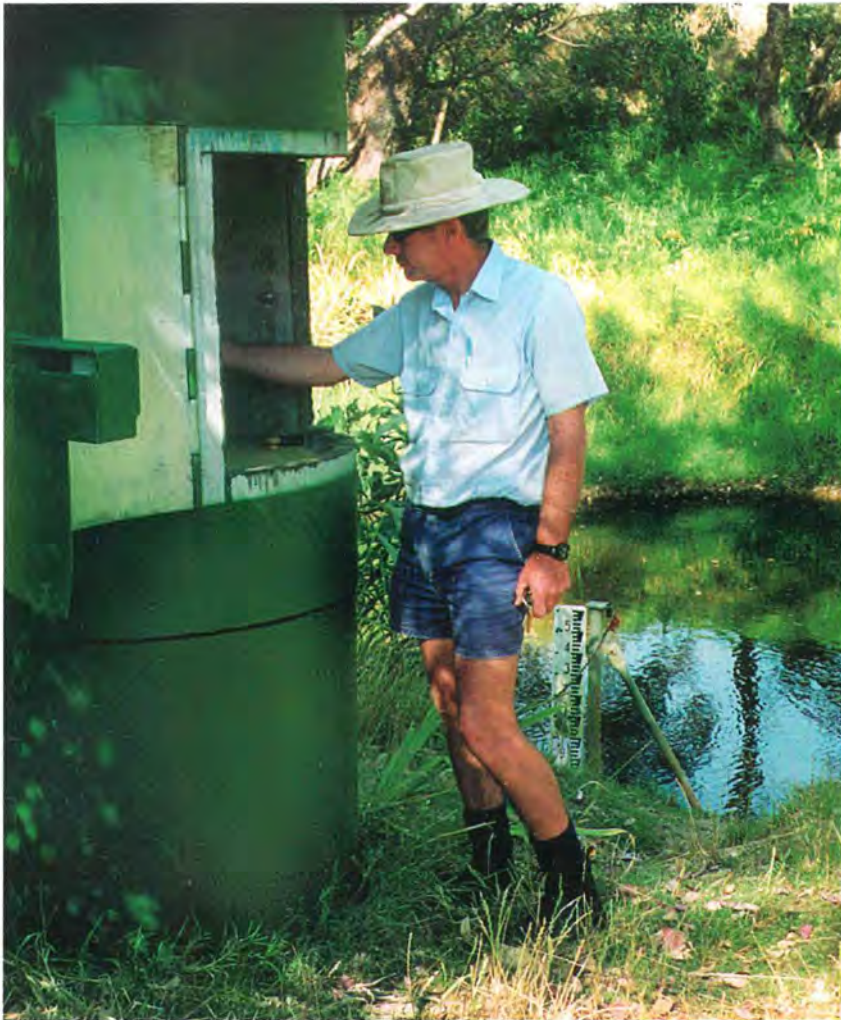
Swan River Trust employee Vaughan Smith taking a flow reading for the Southern River at Anaconda Drive on the Canning Catchment
