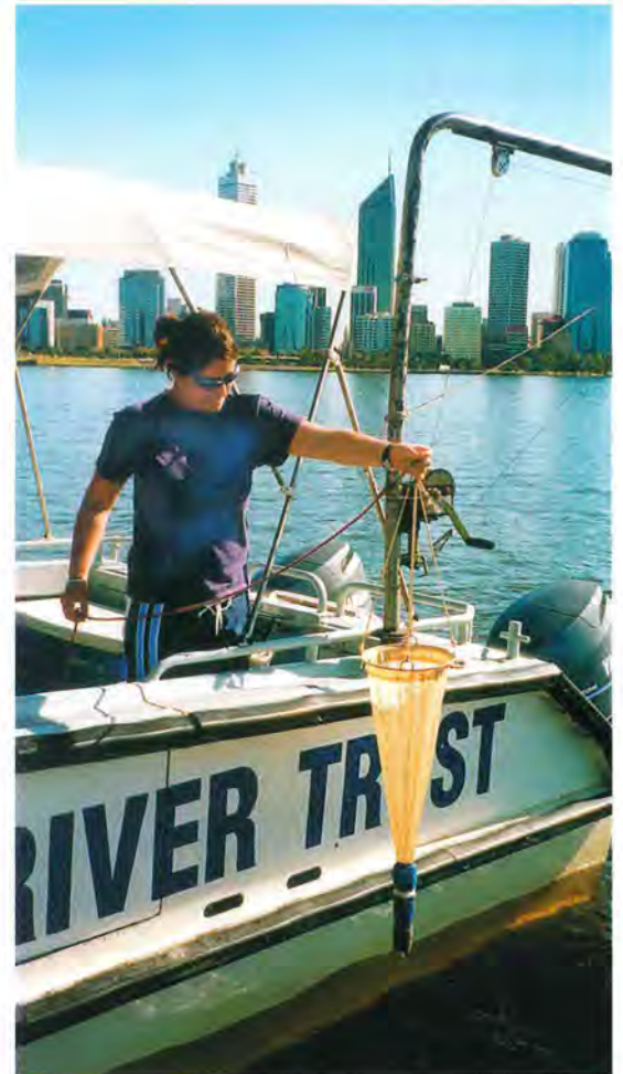
Water and Rivers Commission employee Amanda Wilson taking a phytoplankton sample using a concentrating net
