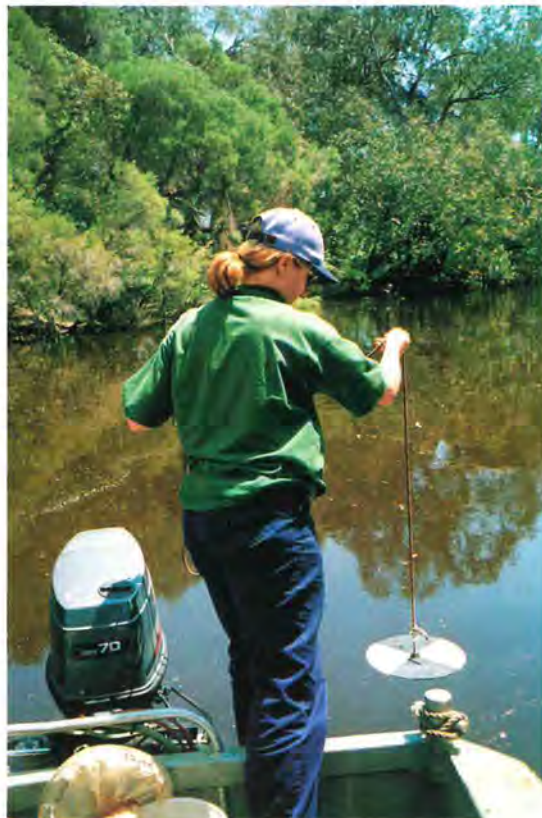
Water and Rivers Commission employee measuring Secchi disk depth on the Canning River
