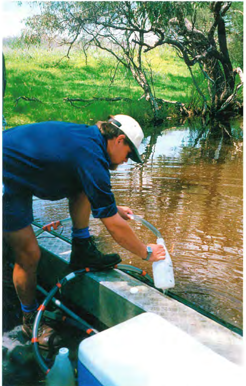
Swan River Trust employee Brian Graco collecting water samples for nutrient analysis
