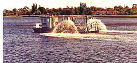
Pumping saltwater from depth and spraying it on Microcystis concentrations to disperse accumulations was also unsuccessful during the bloom in February 2000.
