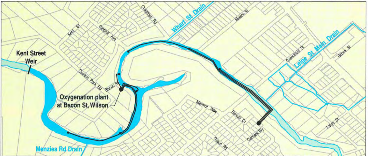
Figure 2: Location of oxygenated area showing location of plants and layout of diffuser pipes
