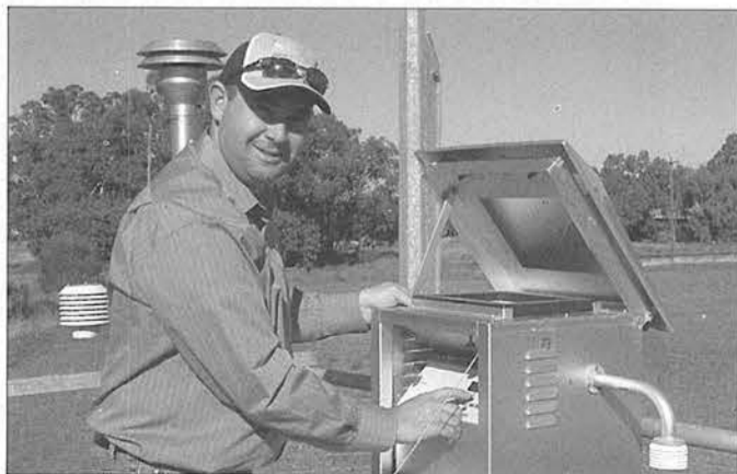
Air Quality Branch Environmental Officer Anthony Horton with a high volume sampler, an active sampler DEC uses to measure total suspended particles and heavy metals. Photo - Nigel Howard
