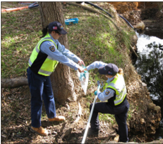
DEC Swan Region Industry Regulation officers Lauren Trott and Maxine Birkin take samples of the leachate in the creek.
