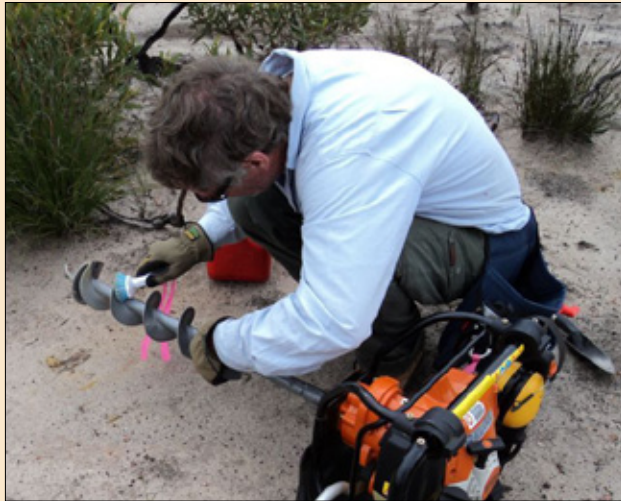
Dr Bill Dunstan, from Murdoch University's Centre for Phytophthora Science and Management, cleaning an auger after assessing the soil profile.
