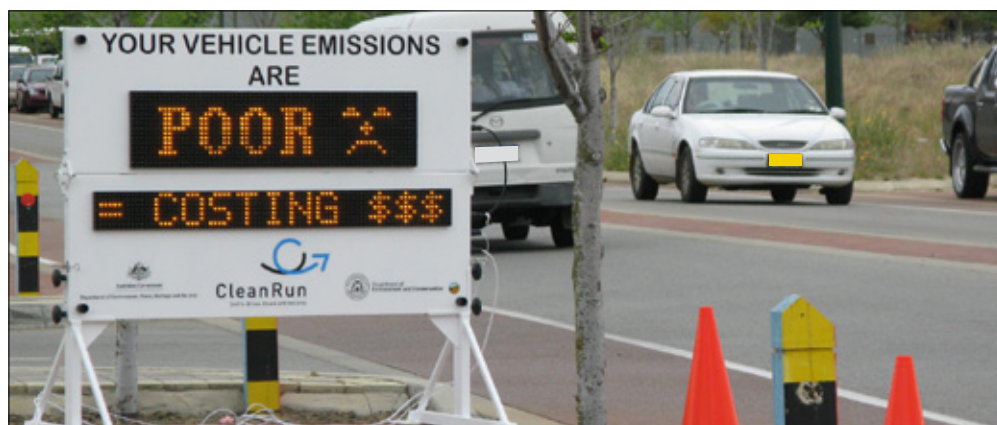
A vehicle travelling on Clayton Street, Midland has just registered 'POOR' on the smart sign, which means their vehicle is producing excessive air pollution and is running inefficiently.
