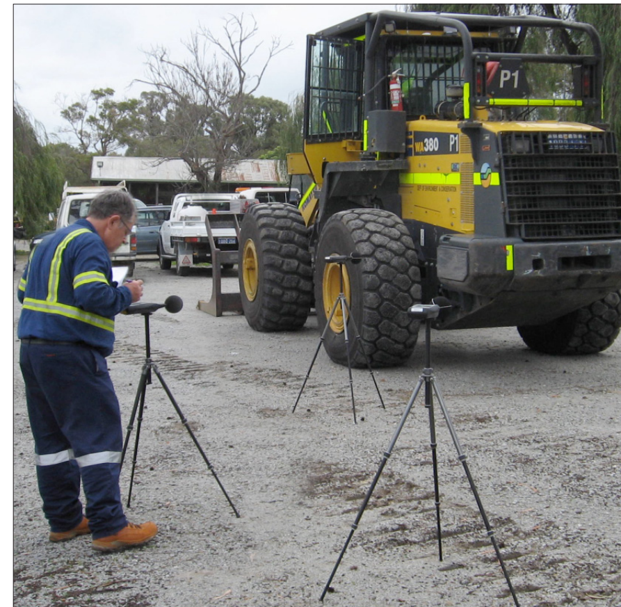
DEC contractor Jonathan Holgate tests the noise output from a broadband alarm.
