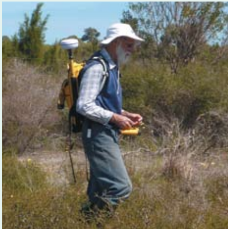
Jim Prince from the Friends of Forrestdale maps weeds using a hand-held computer and differential GPS. Photo – Julia Cullity
