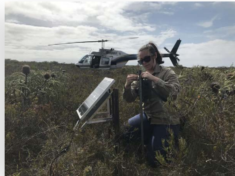
DBCA officer Abby Thomas reinstalling an ARU and solar panel in Cape Arid National Park. Photo – Jeff Pinder.
