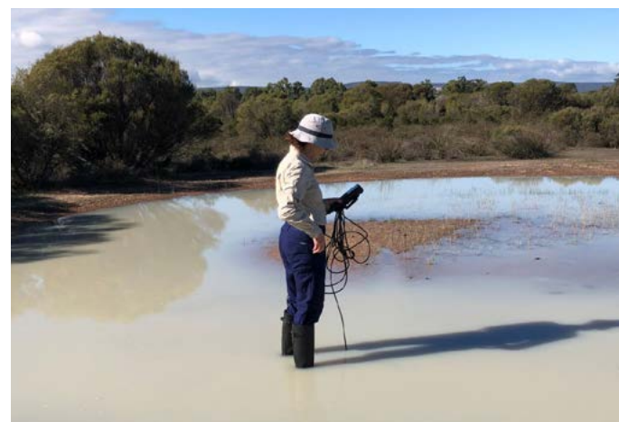
Left: Sampling one of the three groundwater bores at Greater Brixton Street Wetlands. The red coloured groundwater in the bailer shows the presence of dissolved metals such as iron. Right: Sampling surface water using a water quality meter that measures parameters including dissolved oxygen, salinity and pH. Photos – Grazyna Paczkowska.
