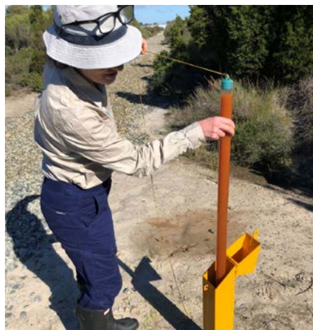
Left: Sampling one of the three groundwater bores at Greater Brixton Street Wetlands. The red coloured groundwater in the bailer shows the presence of dissolved metals such as iron. Right: Sampling surface water using a water quality meter that measures parameters including dissolved oxygen, salinity and pH. Photos – Grazyna Paczkowska.
