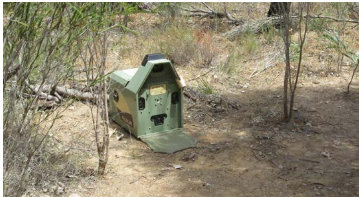
A Felixer grooming trap. These traps are a new technology which use range-finding sensors to recognise cats and foxes, and spray only these target animals with a gel containing the 1080 toxin. Feral cats will groom themselves, licking the gel off their fur and consume a lethal dose of poison. Photo – DBCA.
