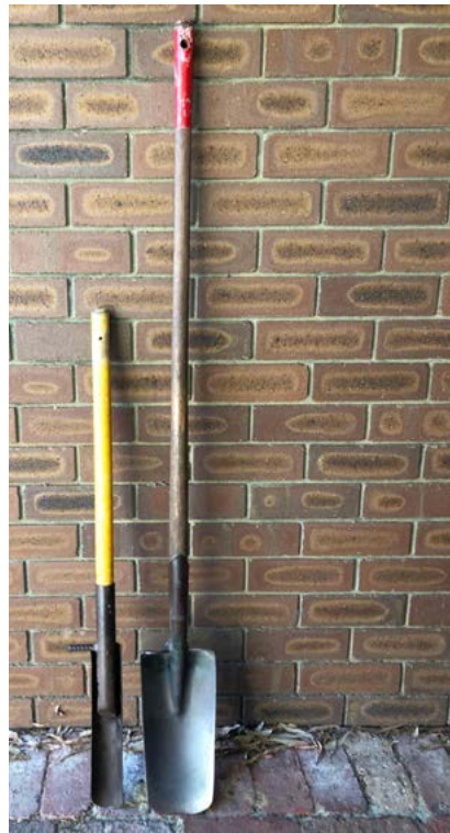
The specially designed half-pipe levering tool (left) and a spade that has had its blade narrowed (right). The narrow blades on these tools make for easier work and less soil disturbance when manually removing weeds such as dune onion weed, sea spinach, pelargonium, Cape tulip and gladiolus from sandy or loamy soils. The half-pipe levering tool is used for removing smaller or bulbous weeds, while the modified spade is used for larger weeds with more extensive root systems. Photo – Mike Norman.
