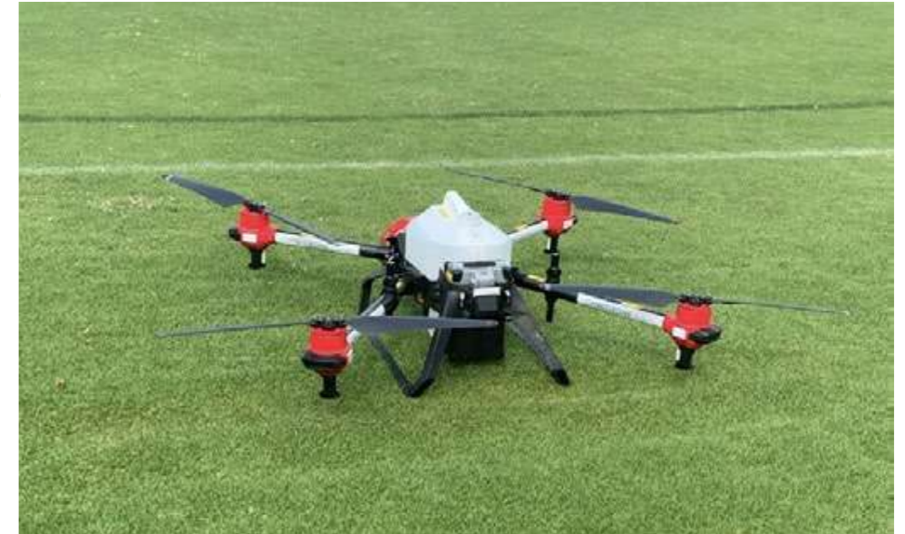
This large commercial drone used for mosquito control weighed approximately 67kg, could carry a payload of 30kg and can treat up to 16ha per hour. Photo –City of Bayswater.
