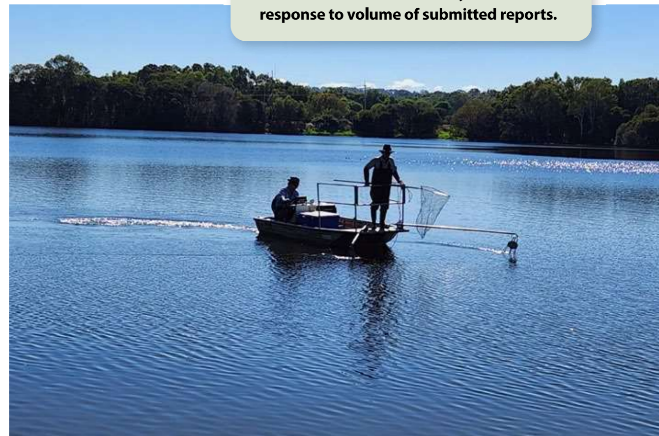
Electrofishing lowers electrodes into the water which causes the fish to swim towards the anode where feral fish are netted and immediately euthanised in an ice slurry. There is no permanent harm to non-target fish. Photo – Jan Saunders.
