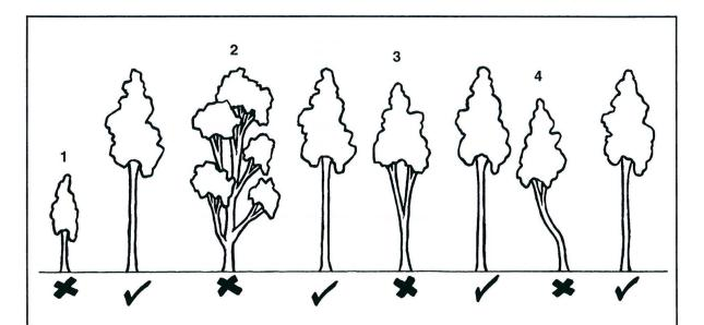
Thinning removes the trees with (1) poor growth, (2) large branches, (3) forks and (4) bent trunks – leaving only the best trees.
