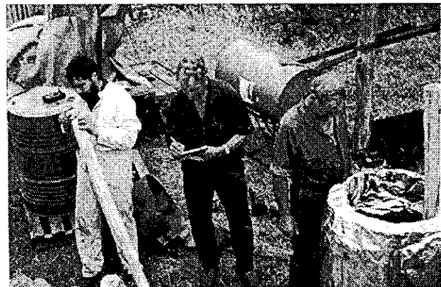
Measuring post and sapwood volume to estimate uptake of preservative.
